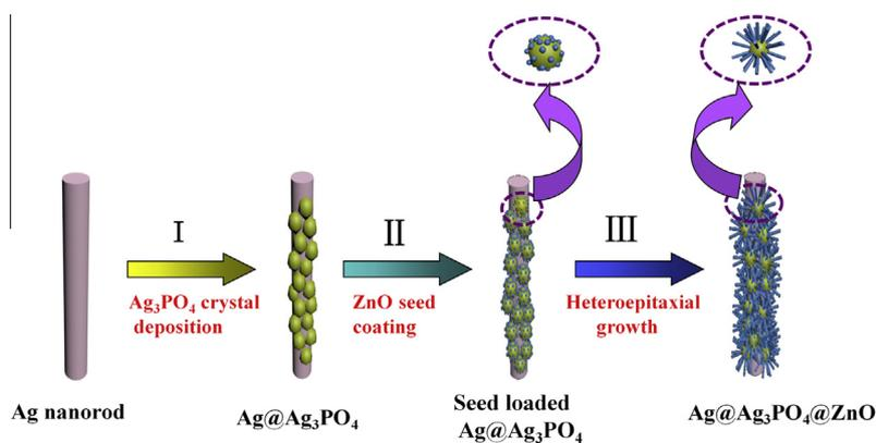
Fig. 1. Schematic illustration of the growth process of Ag@Ag<sub>3</sub>PO<sub>4</sub>@ZnO ternary heterostructures.
